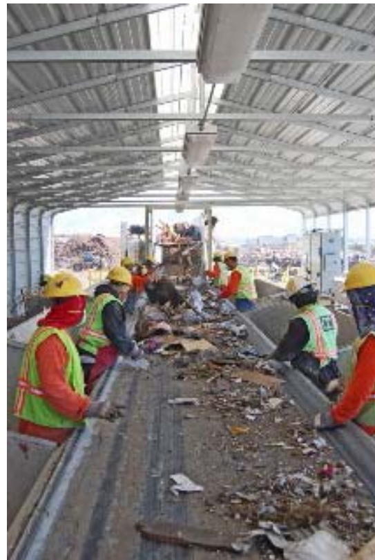
Sorting C&D at Zanker Facility
